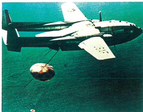
FIGURE 4. AERIAL SNATCHING of a Corona film capsule by a C-119 aircraft near Hawaii. The capsule entered the atmosphere on a shallow trajectory and deployed its parachute at approximately 50 000 feet.
