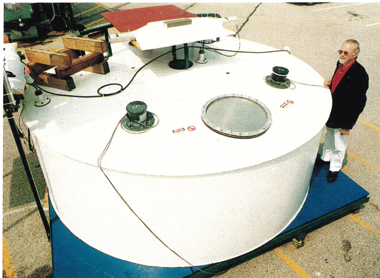
PROTOTYPE ČERENKOV DETECTOR , built at Fermilab for the Pierre Auger Project, contains 12 tons of water monitored by three 8-inch phototubes. Design details are still being optimized by Peter Mazur (right) and colleagues at several collaborating institutions. Each of the project's two air-shower sites will have 1600 such detectors arrayed over 3000 km 2 . Each detector will communicate with a central computer only by solar-powered radio.
