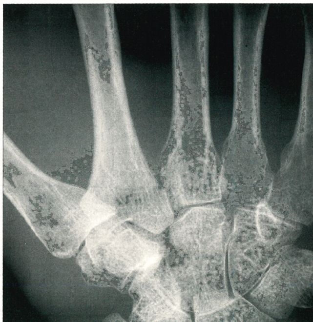
FIGURE 3. AN X-RAY IMAGE OF A PHANTOM HAND obtained using a flat-panel a-Se-based detector.
