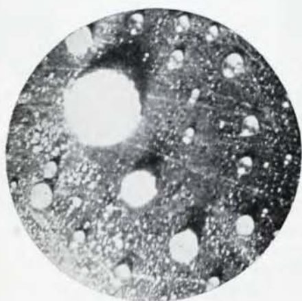
Fig. 9. Water Droplets Freezing on a Cooled Plate.
