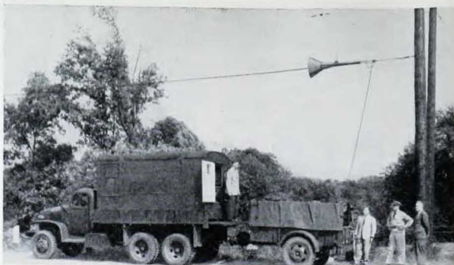
Fig. 6. One terminal of a two-mile experimental surface wave transmission line used by scientists of the Signal Corps Engineering Laboratories. Truck contains equipment for measurement of transmission characteristics.
