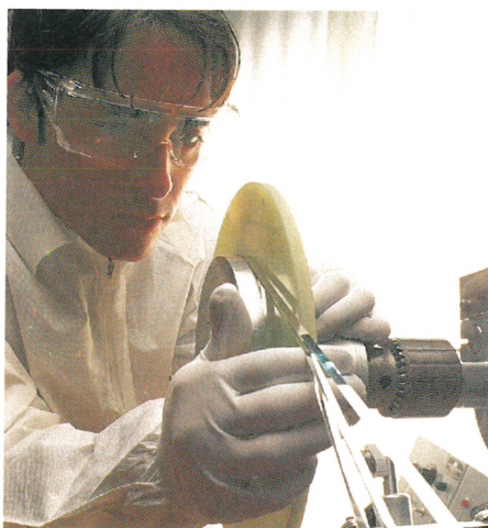
FABRICATION OF A DOUBLE-PANCAKE COIL. It is made of three strands of silver-sheathed Bi-2223 tape (heat treated before winding) and has 37 filaments. (Courtesy of Intermagetics General Corp.)
