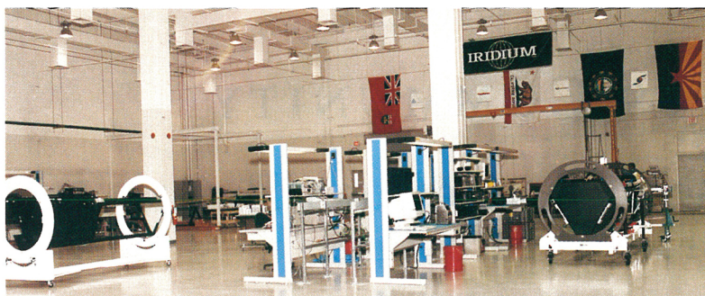
SATELLITES FOR THE IRIDIUM SYSTEM, at left, in various stages of assembly at Motorola's production factory in Chandler, Arizona. (Courtesy of Motorola's Satellite Communications Group.) Below, a depiction of Iridium's satellite-based global mobile telephone system. (Courtesy of Iridium LLC.)
