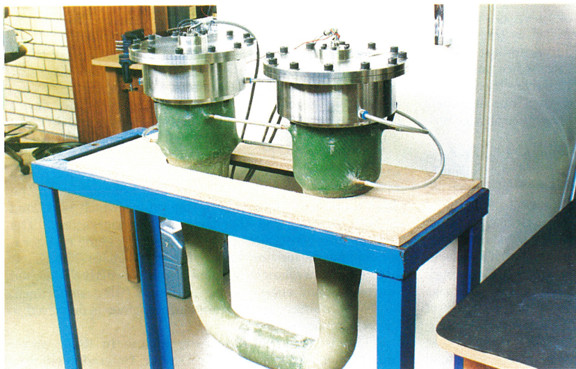
TWO COMMERCIALY INTERESTING thermoacoustic systems. a: Half-wavelength refrigerator with two stacks driven by two loudspeakers was built at CSIR in South Africa. It operates at 120 Hz with 15-bar neon. The heat exchangers are located where the water lines connect to the green resonator body. (Courtesy of Peter Bland, Quadrant.) b: One of the two spiral stacks for the largest thermoacoustic engine to date, being built by Cryenco Inc. (Courtesy of John Wollan, Cryenco.) FIGURE 4
