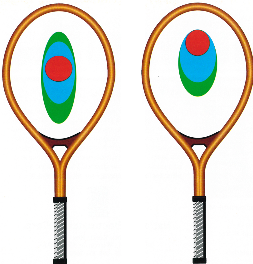
POWER SPOT FOR SERVING a tennis ball is higher on the racket than for a ground stroke, because the effective pivot point of the service motion is very close to the butt end of the racket. For a very stiff, head-heavy racket (right) the power point is higher than it is for a more flexible, neutral-balance racket (left). Successive contours going outward from the optimal power point (red) indicate loci for 99%, 95% and 90% of maximum ball speed. FIGURE 6
