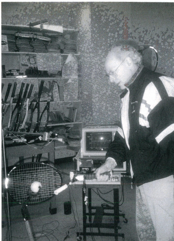
IN HIS LABORATORY at the University of Pennsylvania, Brody examines whether the impact position of a tennis ball can be determined from the magnitude and phase of the resulting racket vibration. FIGURE 2
