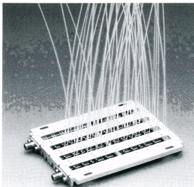
SWITCHED RF FILTER bank produced by Superconductor Technologies Inc for the Air Force has 32 filters in series, uses optical switching of the high- T_c elements to reject unwanted signals, and has three optical fibers per filter.
