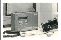
2.2 pounds and measure 7"×5"×2.5". Each unit has eight input channels for thermocouples, thermistors or transducers, plus a pulse-count channel and an 8-bit digital channel that allows eight event inputs. The loggers store up to 65 000 time- and date-stamped readings. Data can be read into a computer, or the readings can be downloaded by modem for remote operation. The loggers run on batteries or ac power. Software is available for statistical and graphical analysis of
