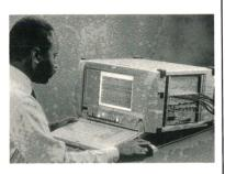
digital converter with a dynamic anti-aliasing filter, and 16 digital inputs. Two independent sample clocks allow the user to acquire both rapidly changing and slowly changing signals. The system can be triggered by such quantities as the input level, input slope, time of day, interval time or an external signal.
