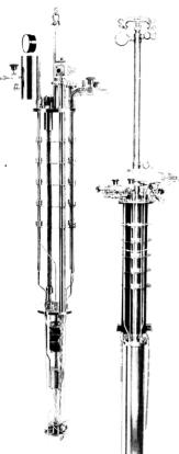
For research applications requiring temperatures down to 0.3 K, Janis Research offers self contained sorption pumped or continuously operating He-3 systems. These systems are designed to hold He-3 from several hours to two days or more.
