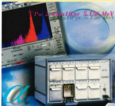
All hardware and software operations are automatically controlled and monitored by a personal computer. Just set up the parameters, start the program and let **OASIS**™ (Oxford Alpha Spectroscopy Integrated System) take over. When you need to change samples, **OASIS**™ automatically controls the vacuum to "active" chambers, stores all information to disk and, if you wish, even prints the results.
