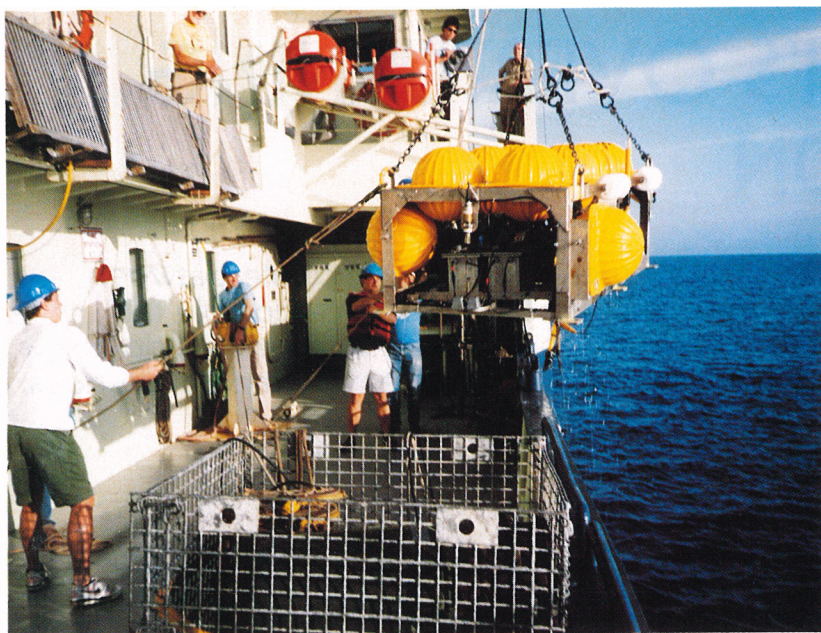
Experiment to measure vertical mixing of ocean waters was conducted by injecting \text{SF}_6 tracer into the Atlantic along a constant-density surface about 310 m deep. After six months the tracer had spread laterally over hundreds of kilometers, but vertically only a few tens of meters—much less than would be necessary to account for the vigor of the ocean's overturning. In this picture the \text{SF}_6 -injection sled is being retrieved aboard the R/V Oceanus, operated by Woods Hole Oceanographic Institution. (Courtesy of James Ledwell, Woods Hole.) Figure 1
