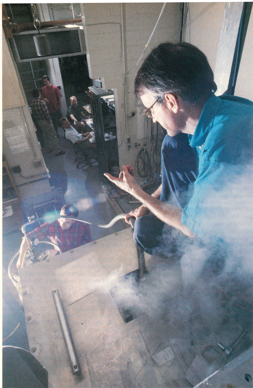
Interdisciplinary research. At Vanderbilt University in Nashville, Tennessee, physics professor John Wikswo (top) and physics graduate student Alan Bradshaw transfer liquid helium into a general purpose SQUID magnetometer, which is housed inside a magnetic shield. In the background are (left to right) physics research associate Daniel Staton, physics graduate student Sergei Rousakov, mechanical engineering graduate student Tony Ewing and physics research associate William Jenks. The "living-state physics" group at Vanderbilt has measured magnetic fields from objects as diverse as human nerves and intestinal smooth muscle, parasites in fish, thin sections of rock, containers of water, samples of Plexiglas, nuclear reactor fuel tubes and sections of aircraft wings. (Photograph by John McDonough; courtesy of Wikswo.)
