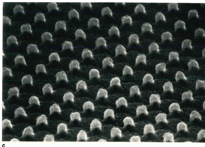
Two ways of making quantum dot arrays at an interface between GaAs (green) and n-doped AlGaAs (red). Both start with an array of photoresist dots serving as a mask. "Deep-mesa-etched" quantum dots (a) are fabricated by etching all the way down into the GaAs, leaving mesas typically 500 nm wide. The potential wells (blue) in which the electrons are trapped near the interface are narrower than the mesas. A field-effect array (b) is made by depositing a semitransparent metal gate (purple) on the photoresist mask (yellow). Voltage applied between the gate and a semitransparent contact layer (between dashed lines) in the GaAs concentrates the interface electrons into potential wells where the gate is farthest away. A scanning electron micrograph (c, below) of a field-effect quantum dot array in an InSb structure 3 shows photoresist dots 100 nm wide covered by a metal gate layer. Figure 2
