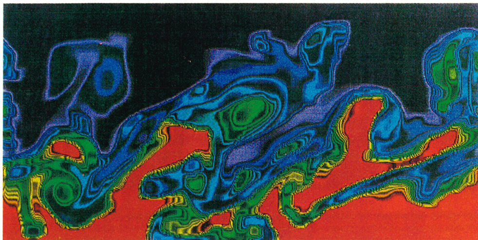
Supersonic streams of counterflowing, chemically reacting hydrogen and air simulated by flux-corrected transport on the CM-2. Color indicates hydrogen mole fraction: Deep red represents pure hydrogen; deep purple, pure air. The lower flow is moving from left to right. (Courtesy of Patrick Vuillermoz, ONERA; and Elaine Oran, Naval Research Laboratory.)
