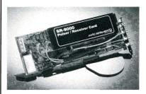
100-MHz bandwidth and a dynamic range of 63.5 dB, the SR-9000 can nondestructively evaluate electronic, structural and biomedical materials and components for latent defects. The card's utility software lets the user control all functions, including pulser damping, repetition rate, output level, rectification, receiver gain and signal filtering.
