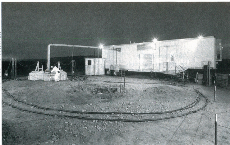
Mobile unit for in situ vitrification of underground waste. PNL is developing this technology, in which electrodes are implanted in the ground, heating it to high enough temperatures that the soil, and the waste it contains, is fused into a glass-like form.
