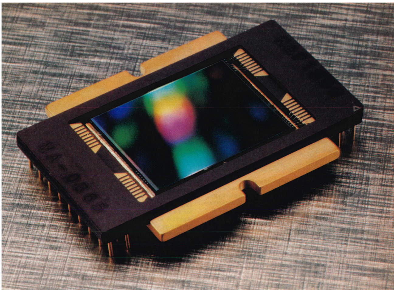
Charge-coupled device with 1.3 million pixels. The photosensitive surface of this full-frame imager is 20.5 \times 16.4 mm. Each pixel is a square, 16 microns on a side. (Courtesy of Eastman Kodak.) Figure 1
