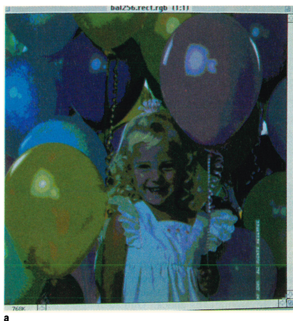
Digital color image displayed with 256 colors that were selected from a set of 16 million colors to produce either an image-independent palette (a) or an image-dependent palette (b). The palette for a was obtained by uniformly sampling the RGB color space. For b, by contrast, the palette is made up of colors that are common in the image. (Original image courtesy of Eastman Kodak.) Figure 5
