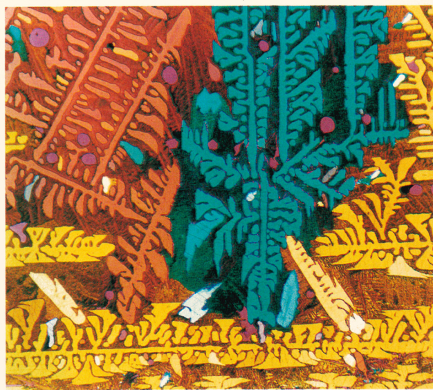
Dendritic microstructures. Left: Micrograph of a cast Cu-Zn alloy (commercial 70/30 brass). In this sample, etched to show its microstructure, the dendrites solidified first, leaving impurity-rich liquid to solidify later in the interstices. The region swept out by each primary dendrite and its array of sidebranches is (very nearly) a single crystal, or grain, whose symmetry and orientation are the same as those of the dendrite. Thus, the dendritic mechanism determines both the grain structure and the patterns of chemical composition within the grains. (Courtesy of J. P. A. Löfvander, University of California, Santa Barbara.) Above: Solidification pattern obtained by quenching a thin film of an initially uniform mixture of two molten salts, CuCl and PbCl 2 . The PbCl 2 -rich crystals are dendritic. Because the photograph was taken through crossed polarizers, the birefringent PbCl 2 crystals appear as brightly colored regions, each color corresponding to a different crystalline orientation. (Courtesy of J. van Suchtelen, Philips Research, Eindhoven, The Netherlands.) Figure 1
