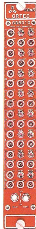
For adjusting the delay and width of coincidence and gating pulses
