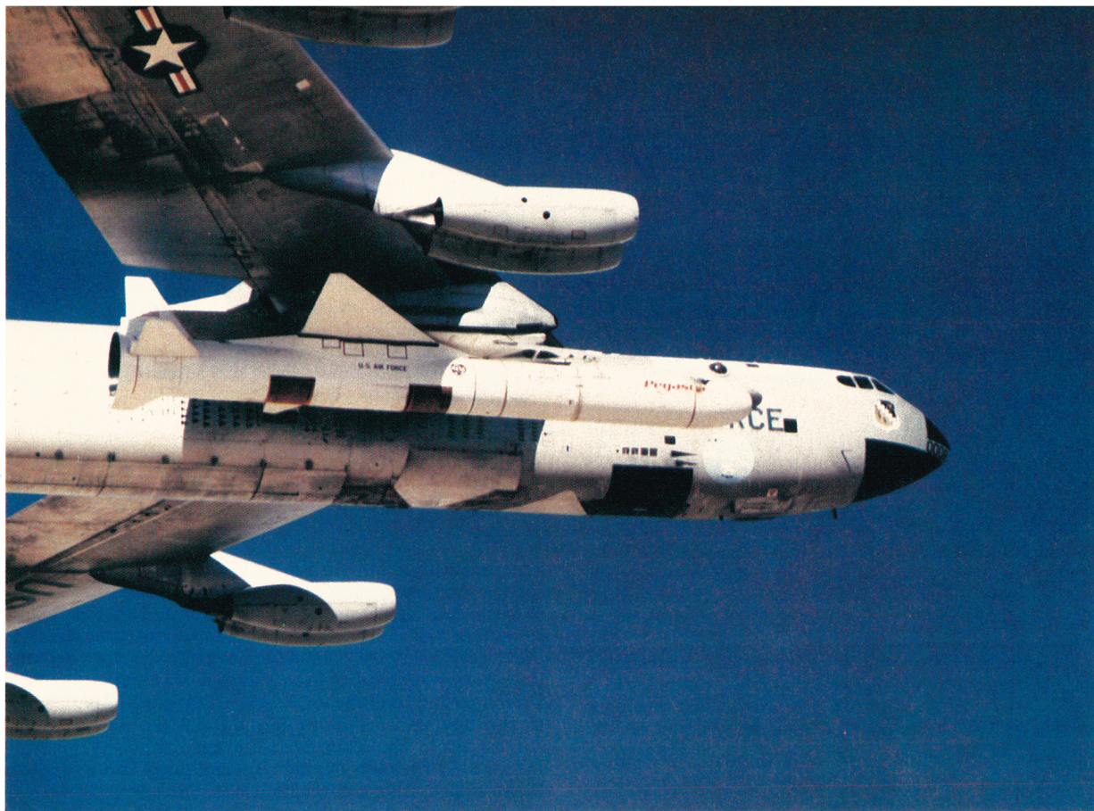
Small expendable launch vehicle. All but the first mission in the Small Explorer Program are scheduled to fly on airplane-launched winged Pegasus rockets like the one shown here. Figure 1
