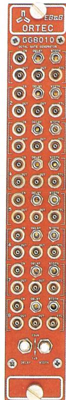
For adjusting the delay and width of coincidence and gating pulses
