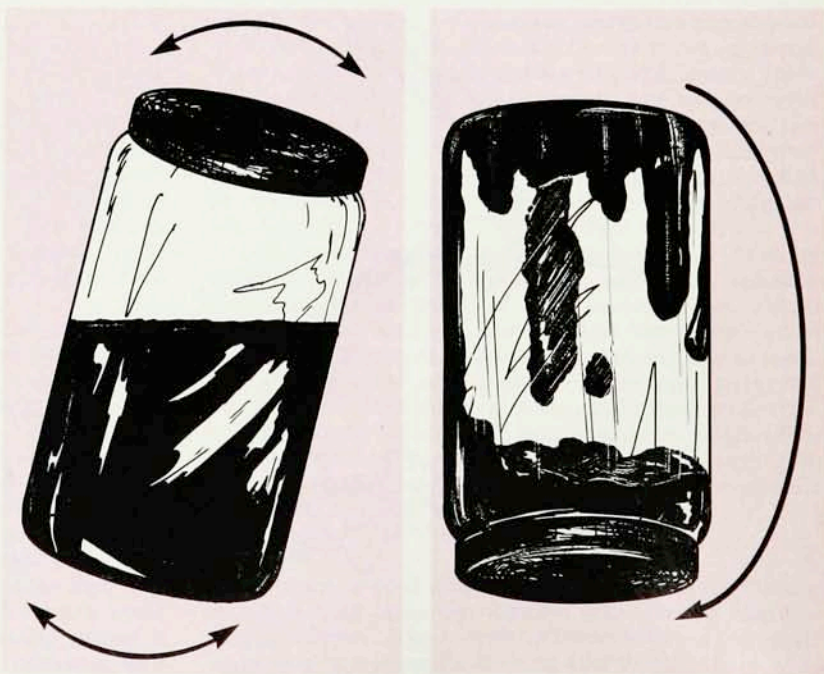
Solutions of associating polymers have moderate viscosity values in a state of gentle flow (left). But such a solution gels under the application of shear, as when a jar containing it is rapidly inverted (right). Figure 5
