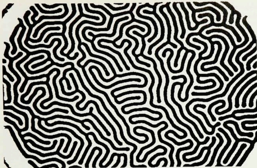
Labyrinthine pattern formed by a drop of ferrofluid between two horizontal glass plates about a millimeter apart, when the plates are inserted between the poles of a magnet, normal to the magnetic field. As the magnitude of the field increases from zero, the initially circular droplet breaks into spikes, which elongate and branch out to fill the area between the plates. The thickness of the ferrofluid channels (black) is comparable to the spacing between the plates. 3 (Courtesy of R. E. Rosensweig, Exxon Research and Engineering Company. Figure 2 )
