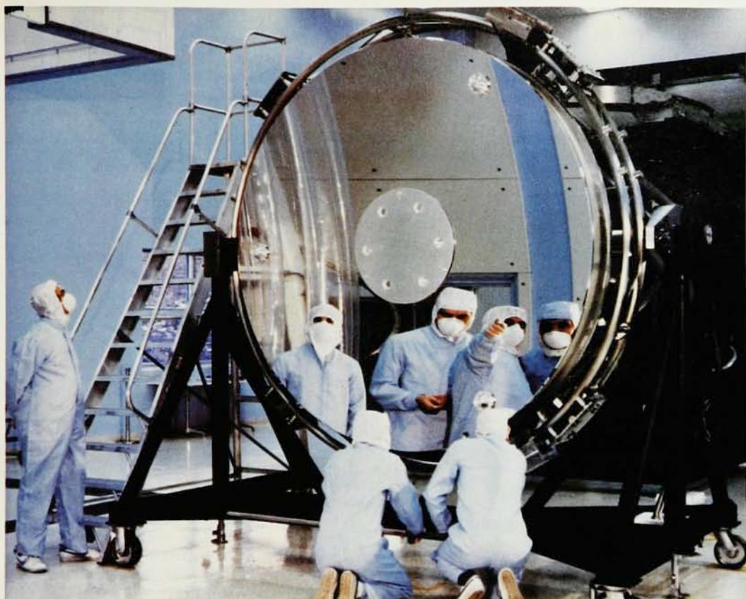
The optical performance of the HST's mirror exceeds NASA specifications. Reflective coating is aluminum because it absorbs little uv. The three circles at approximately 1, 5 and 9 o'clock on the mirror are hoist-bolt locations.
