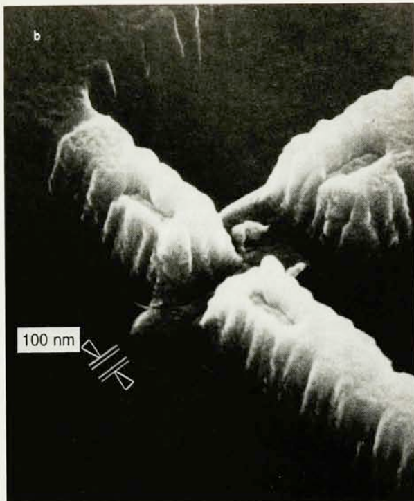
MOSFET schematic diagram (a) and micrograph (b). The cross-sectional schematic is of a silicon transistor with a 100-nm channel length, part of a ring oscillator circuit fabricated using electron-beam lithography. To make the electron micrograph, the contact metal and oxide were removed. The two structures that go diagonally across the image from upper left to lower right are the source and drain contacts; the gate is in the gap between them. The switching times of such short-channel silicon transistors are competitive with those of field-effect transistors made with III-V semiconductors. (Micrograph courtesy of T. H. Philip Chang and Dieter P. Kern, IBM.) Figure 3
