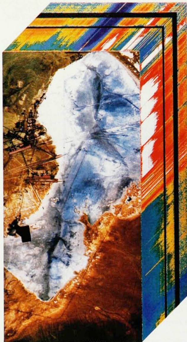
Hyperspectral image of Rogers Dry Lake in California, taken by AVIRIS. The lake bed is shown in a false-color composite, in which red represents a wavelength of 0.690\ \mu\text{m} ; green, 1.534\ \mu\text{m} ; and blue, 2.222\ \mu\text{m} . The runways at Edwards Air Force Base are clearly visible at the left, extending onto the lake bed. The multicolored strip seen in perspective shows the complete spectra of the pixels along two edges of the rectangular image. Moving "into the page," the wavelengths are increasing, from 0.4\ \mu\text{m} to 2.45\ \mu\text{m} . The black bands in the spectra of the edge pixels show the atmospheric \text{H}_2\text{O} absorption at 1.4 and 1.9\ \mu\text{m} . (Courtesy of Gregg Vane, NASA and the Jet Propulsion Laboratory.) Figure 7
