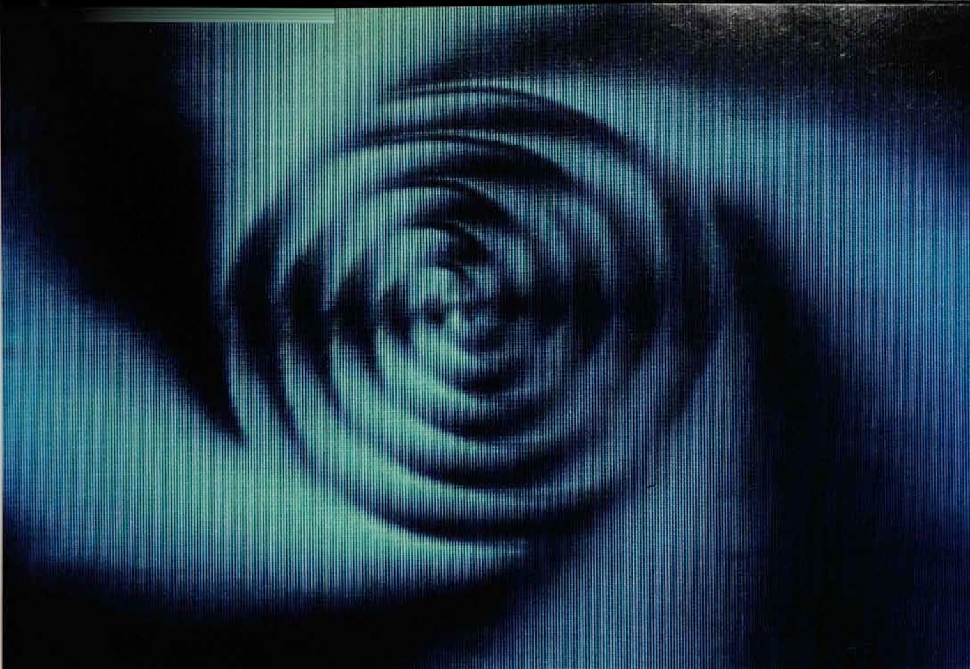
Spiral star defect in a three-layer film of the liquid crystal (S)-4-(2'-methylbutyl)-phenyl-4- n -octylbiphenyl-4-carboxylate in the chiral S_1 phase just below the S_C - S_1 transition. (Courtesy of Steven Dierker, AT&T Bell Laboratories.) Figure 1
