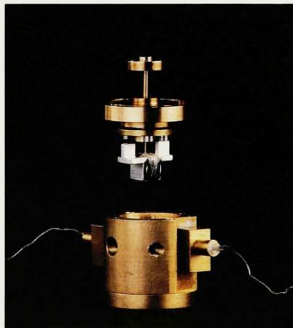
Torsion oscillator used at Cornell to measure the superfluid density. The torsion rod is attached at the top to a flange, which attaches the cell to a cryostat, and at the bottom to a 1-inch-diameter collar, which attaches the oscillator to "massive" cup (shown at bottom) that acts as a vibration isolator. A second, 20-mil-diameter hollow torsion rod (silver) is used to fill the sample cup with helium. The oscillator is driven electrically. The blocks around the sample cup are the drive and detector electrodes. (Photo courtesy of John D. Reppy.)
