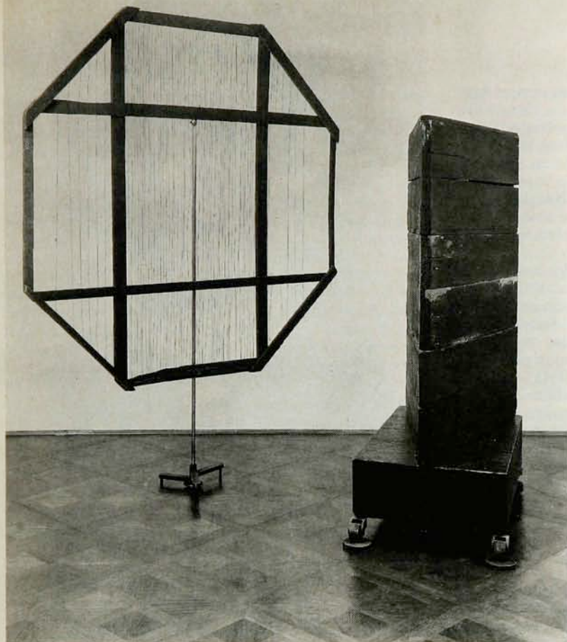
Apparatus that Heinrich Hertz used to study the polarization and refraction of electromagnetic waves. The wire frame, almost 2 m high and strung with parallel wires, acted as an analyzer for the polarized radiation produced by Hertz's spark transmitter. The 30° prism, when filled with hard pitch, weighed more than 1000 lbs. (Courtesy of the Deutsches Museum, Munich.)
