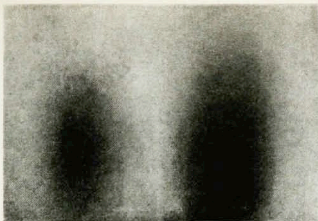
N rays could enhance illumination of a dimly lit object, or so Blondlot claimed. Among other evidence, he published the above photogravure, made by exposing film to a small luminous spark. The darker exposure (right) was made in the presence of N rays, mysterious radiation emanating from a hot wire. (From Comptes Rendus , 22 February 1904.)
