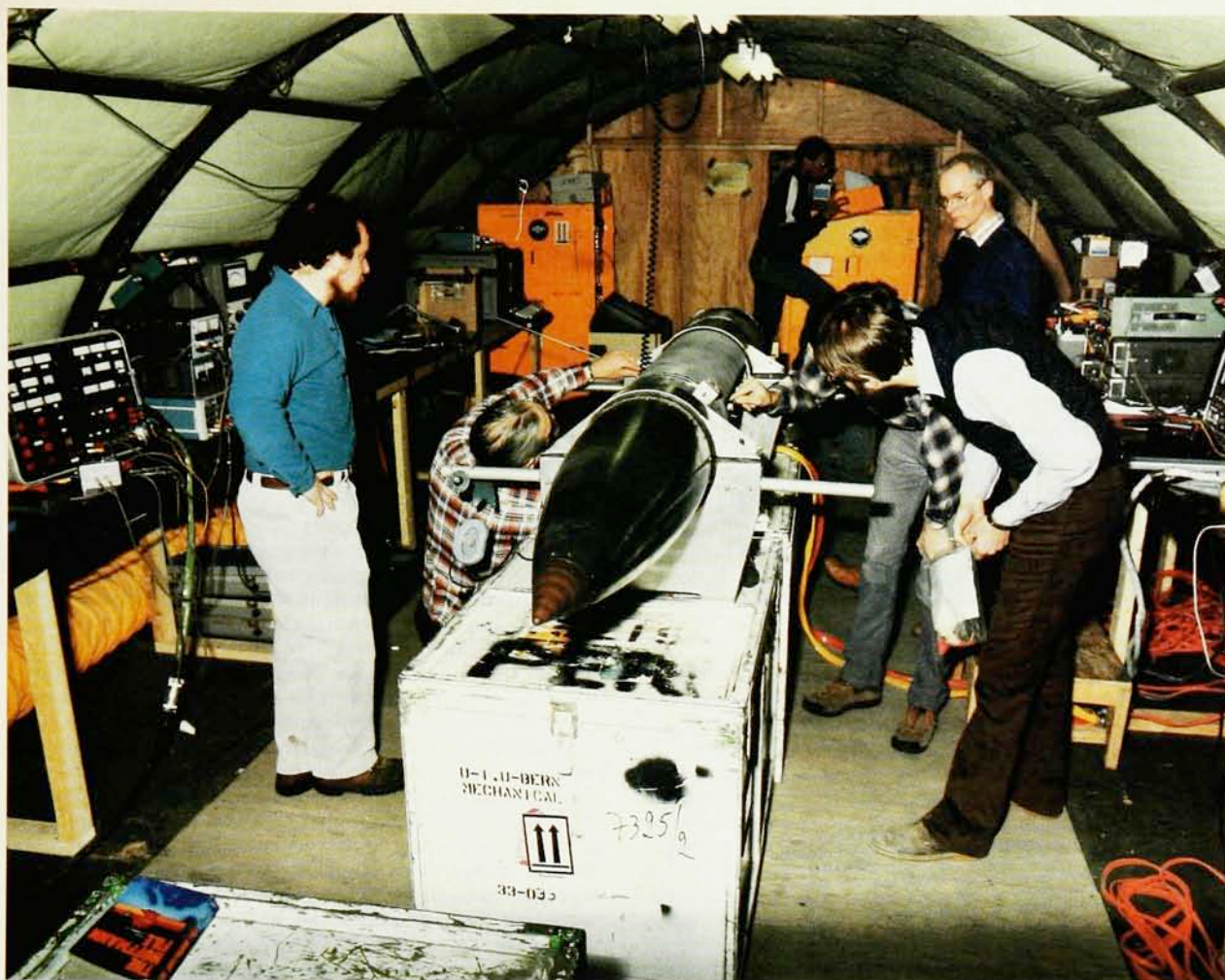
Suborbital rockets are essential for carrying instruments to study auroral plasma physics—for example, to measure ion acceleration processes. Here a payload is undergoing checkout at the launch site prior to launch on a three-stage Black Brant 10 rocket from Søndre Strømfjord, Greenland. The instruments were built by scientists from the University of New Hampshire, Cornell University, Marshall Space Flight Center and the University of Bergen, Norway.
