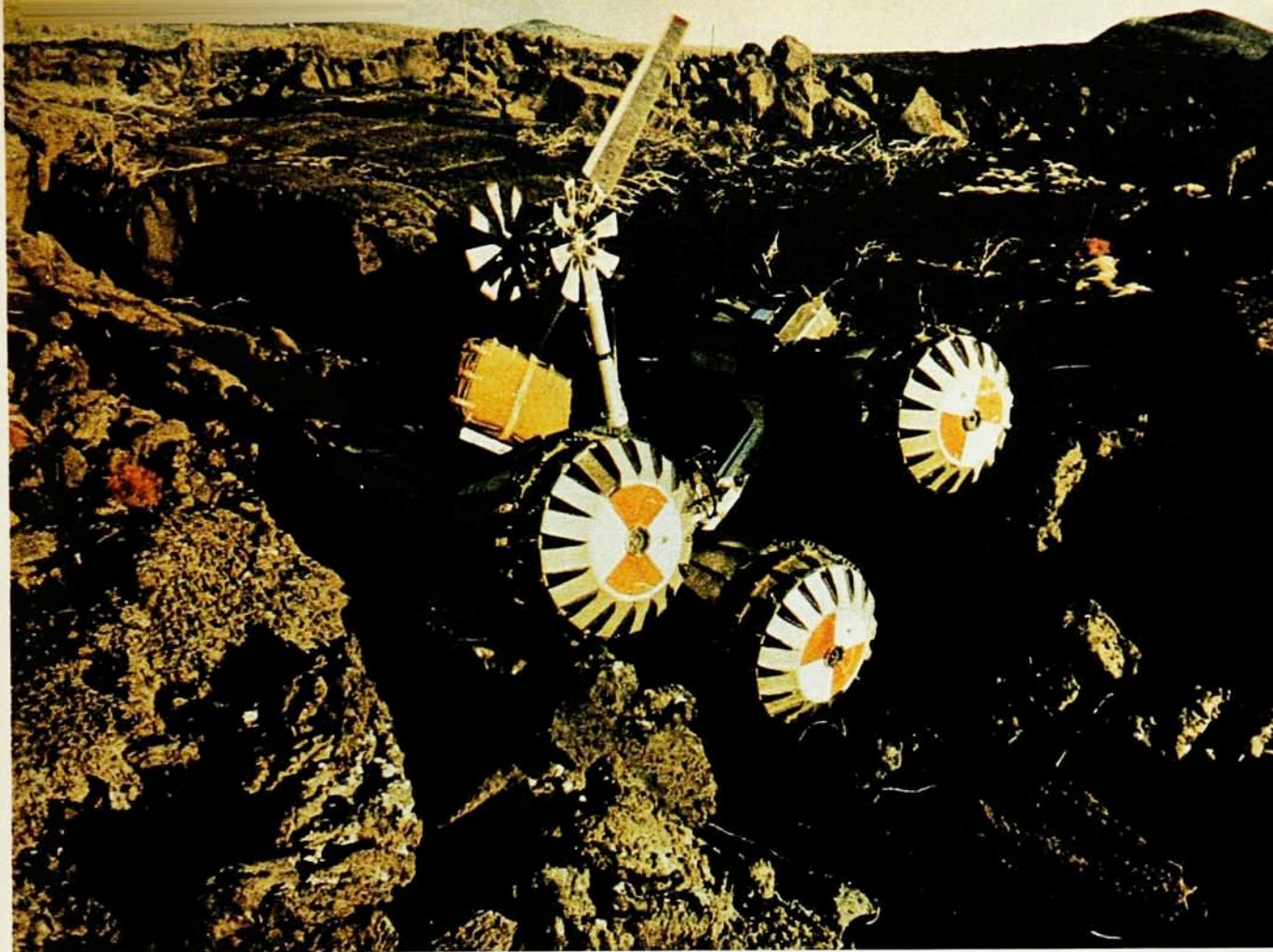
Mars rover during testing. The small vehicle is under development for a mission to the planet in 1994. It would travel several tens of kilometers and would sample soil to depths of several meters. Figure 1
