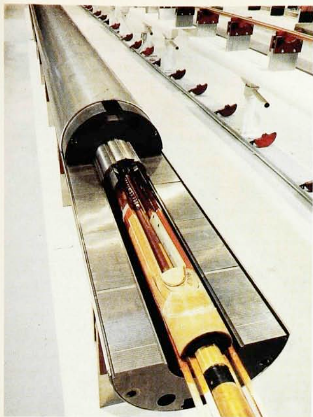
Superconducting coil end of a full-length SSC test magnet at Brookhaven National Laboratory is visible in this photo because the last few feet of laminar collar and surrounding laminar yoke have not yet covered the inner and outer upper coils. Where they make their U turns at the coil end, the superconducting cables experience enormous longitudinal Lorentz forces tending to stretch the 17-meter-long coil. The SSC magnet program is investigating various ways of preventing these forces from causing premature quenches. When the yoke and outer skin are complete, the magnets are installed in their cryostats at Fermilab and tested at liquid helium temperatures. (Photo courtesy of Brookhaven.)
