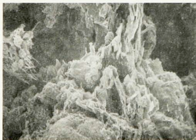
Sandstone as seen with an electron microscope. a: A 2.5-mm-wide region of a sample from Fontainebleau, France. b: A 0.05-mm-wide region of the same sample. c: Illite clay in a Coconino sandstone, at about the same magnification as in b . Figure 2
