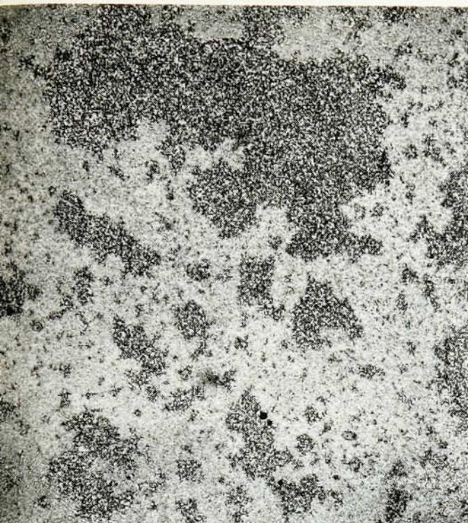
Percolation of air through paraffin oil in a 350 \times 350 network of randomly sized grooves etched into a glass plate. 20 At a sufficiently slow flow rate, the oil is displaced pore by pore through the invasion percolation mechanism. The light area is the air, which forms a connected path across the sample. The dark regions are immobile, disconnected patches of trapped paraffin oil. Such trapping is a major cause of low oil recovery from a reservoir. (Photograph courtesy of R. Lenormand, Dowell-Schlumberger.) Figure 6
