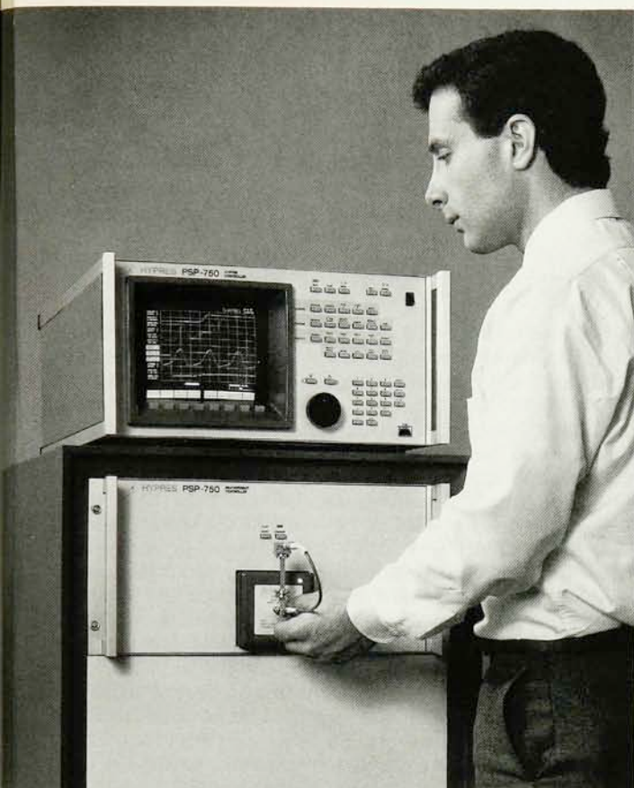
Oscilloscope developed and marketed by Hypres uses Josephson junction electronics for high-speed sampling. The oscilloscope has a bandwidth of 70 GHz, which is more than three times larger than the bandwidth of a typical nonsuperconducting oscilloscope. Hypres is based in Westchester, NY. (Courtesy Hypres.)
