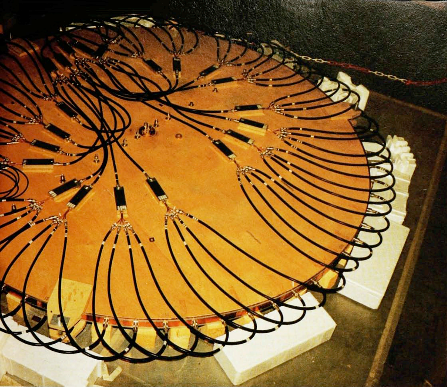
Scale model radial transformer line for the switched-power linac scheme, built at CERN to study transformer ratio as a function of pulse length. A transformer ratio of more than 20 was observed, in good agreement with theory, and not sensitive to drive imperfections. Figure 4
