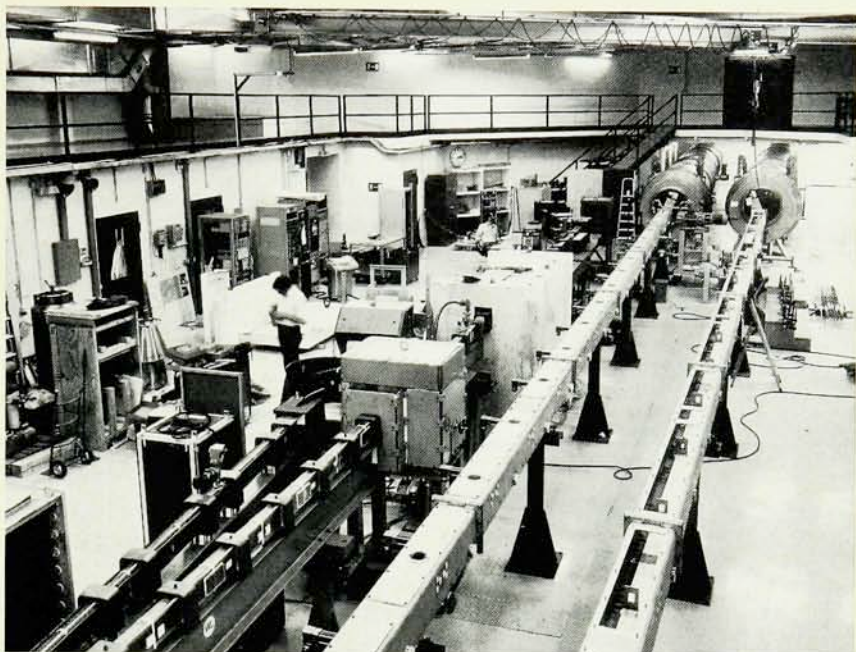
New cold-neutron guide hall at the Jülich Nuclear Research Facility is seen here from the vantage point of the reactor building. In the upper right-hand corner of the photograph are two small-angle neutron scattering instruments, which are to be used in metal physics, polymer research and biology. To the left, two small neutron guides deliver neutrons to a triple-axis spectrometer and a nuclear spin resonance apparatus.
