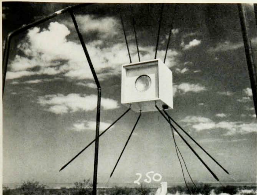
Loudspeaker used to record the arrival of the sound wave and of the shock wave from the first nuclear explosion. Ten such loudspeakers were used to measure the shock wave's velocity.
