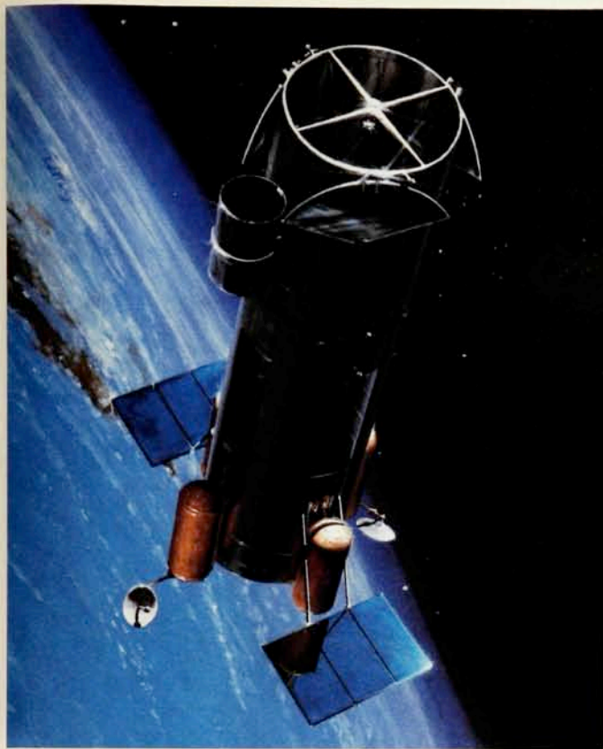
High-power chemical laser battle station in a low Earth orbit is portrayed in this artist's conception. Their comparatively compact power sources make chemical lasers favorable for space basing. Their long wavelengths necessitate using large optics over very long ranges. Atmospheric absorption makes these lasers unsuitable for ground basing.
