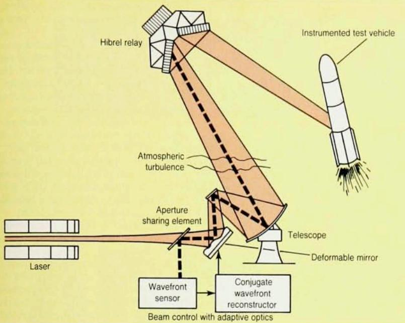
**Schematic drawing** showing how adaptive optics (pictured in figure on facing page) could be integrated into a ground-based laser system. A downlink signal from the relay mirror, passing through the turbulence, tells the wavefront sensor how to cancel the atmospheric effects. A computer reconstructs the wavefront that will perform the compensation and drives the actuators that deform the rubber mirror segments by the precise amounts required.
