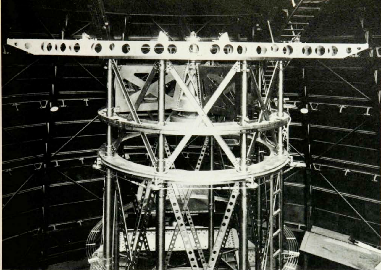
Stellar interferometer that Michelson used in 1920 to make the first measurement of a star's diameter. (Courtesy of William Osborn, Case Western Reserve University.)
