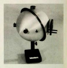
has high spectral reflectance and nearperfect diffuse reflectance, for a usable wavelength range of 200-2500 nm.
