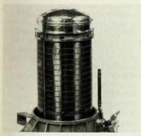
others. The cooling power of the ventline gas is conducted in a controlled manner throughout the length and circumference of the radiation shield. The result, we are told, is a superior hold time with negligible weight pen-
