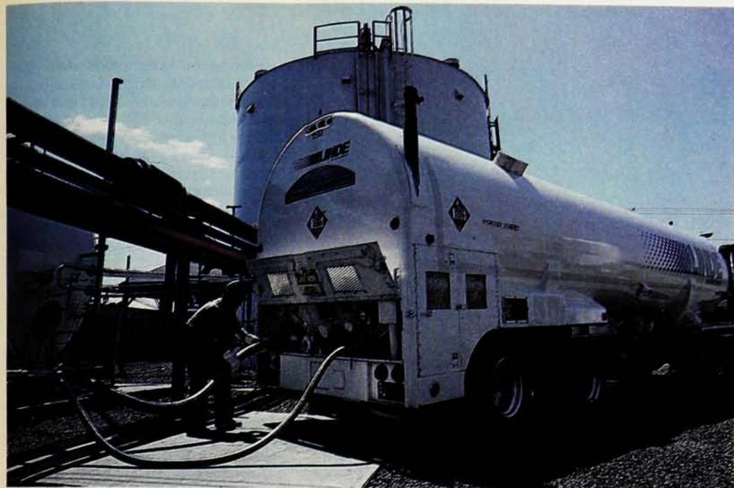
Truck with a tank capable of holding 10 000 gallons of liquid hydrogen or liquid helium for extended periods without appreciable loss. Superinsulation and liquid nitrogen jacketing limit losses to 50 gallons per day. (Photo courtesy of the Linde division of Union Carbide Corporation.)
