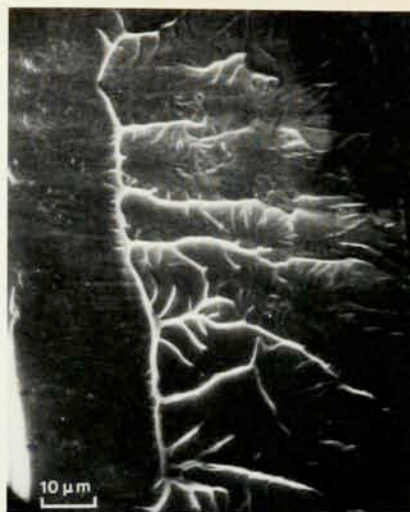
Scanning electron micrograph of the fracture surface of an amorphous metal ribbon broken in the ductile fracture mode. The illustration appears with an article on metallic glasses in the Encyclopedia of Materials Science and Engineering , reviewed here.
