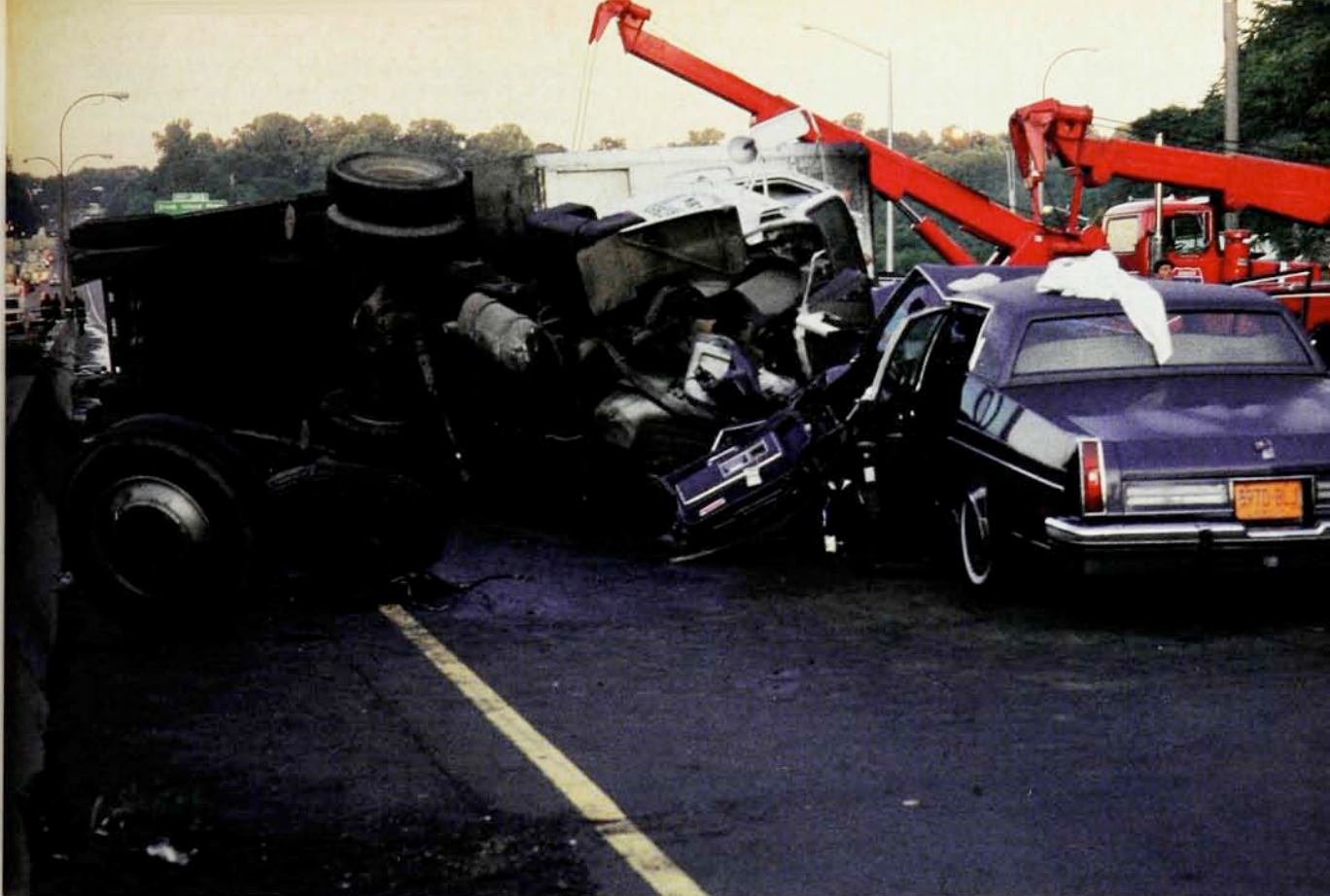
Vehicle-vehicle collision. The tractor-trailer truck crossed the concrete median barrier and collided head-on with the car. The truck's center of mass was higher than the barrier. (Photograph by Richard A. Retting, New York City Department of Transportation.) Figure 1
