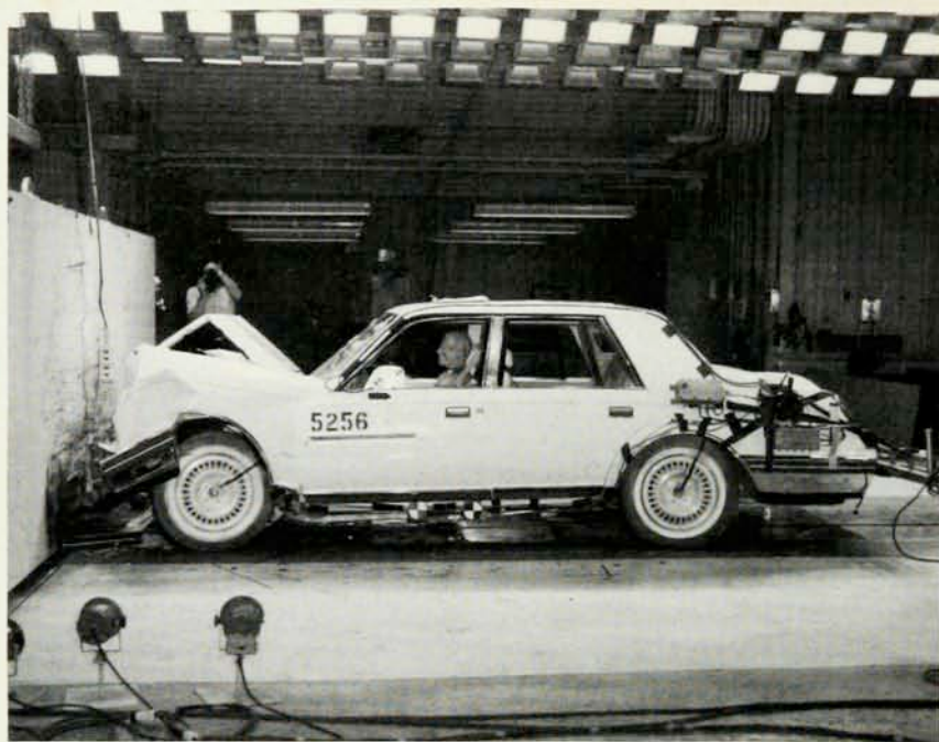
Car-barrier collision test. Dummies in such tests are wired with up to 70 accelerometers. (Courtesy of Ford Motor Company Auto Safety Center.)
