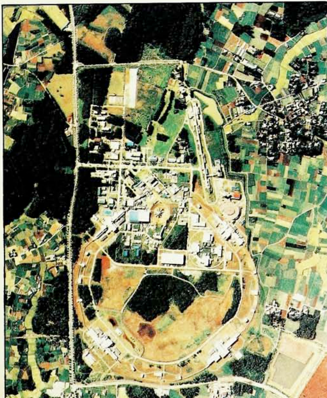
Aerial view of Tristan site in Tsukuba, Japan. The 400-meter linac injects 2.5-GeV electrons and 2.5-GeV positrons into the main ring, whose circumference is 3018 meters. In the main ring the electrons and positrons are each accelerated to 25 GeV and allowed to collide.
