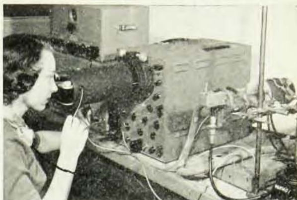
Figure 6. NBS scientists are using this specially designed apparatus for studying the internal friction of crystals. From measurements of the decay of free torsional oscillations of a composite piezoelectric resonator it is expected that the effects of crystal imperfections on semiconducting properties will be revealed.
